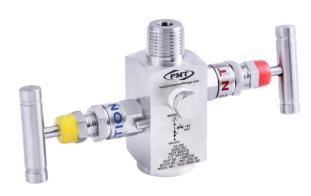
**PMT** 2 Valve Remote Mount manifolds are designed in such a manner, which helps in connecting system impulse line & transmitters. Our range of manifold consist two valve configuration which allows for easy isolation, calibration, block and bleed for gauges, pressure switches and static pressure transmitting instruments.
