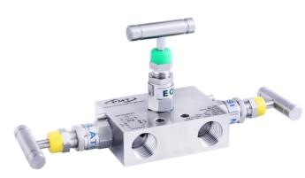
**PMT** 3 Valve Flange to Flange Manifold are Designed for direct or remote mounting of differential pressure Transmitters. For remote mounting two oval / kidney flanges are used for connecting process pipe to manifold block. The manifold block incorporate two main valves for process isolation and one valve for equalizing.
