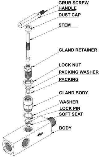
**GRUB SCREW**: For locking the handle.
