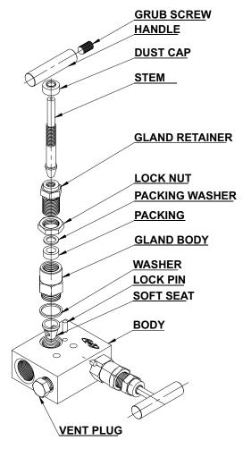
**SOFT SEAT**: PTFE & Delrin Seat to ensure a tight-shut off even in abrasive process conditions.
