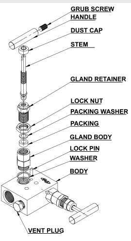
**BODY**: Forged one piece body construction (no welding) for high strength.
