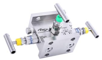
**PMT** 3 Valve Flange to Flange Manifold are Designed for direct or remote mounting of differential pressure Transmitters. For remote mounting two oval / kidney flanges are used for connecting process pipe to manifold block. The manifold block incorporate two main valves for process isolation and one valve for equalizing.
